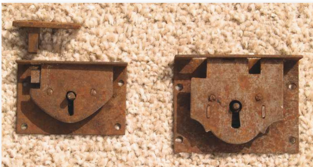
Two early 18th-century steel locks; the one on the left has a link plate
